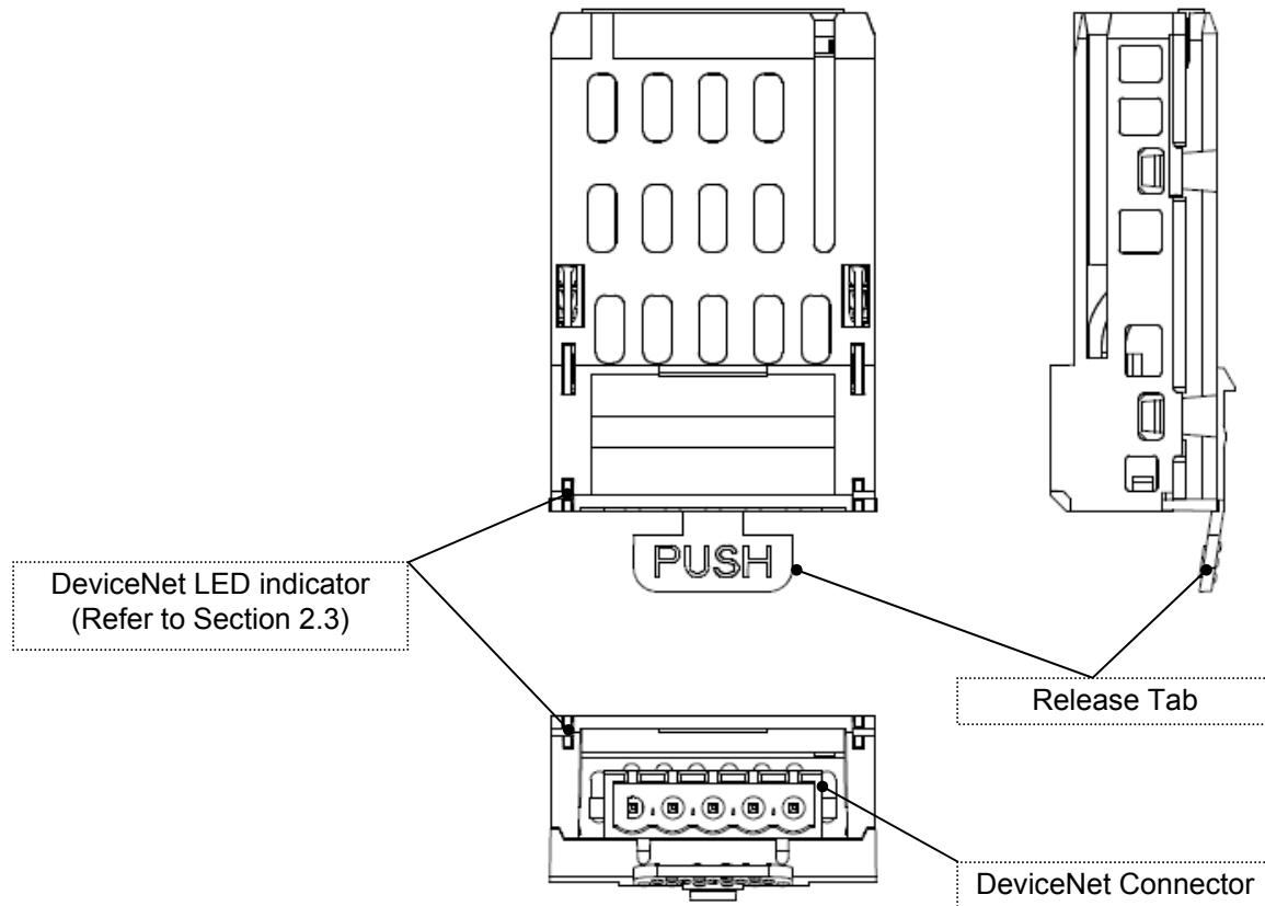
Multi-Drop type connector etc. can not be used for DEV003Z.
